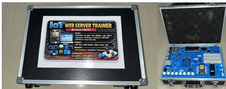
Figure 5. Physical Prototype of the Web Server-Based IoT Trainer
